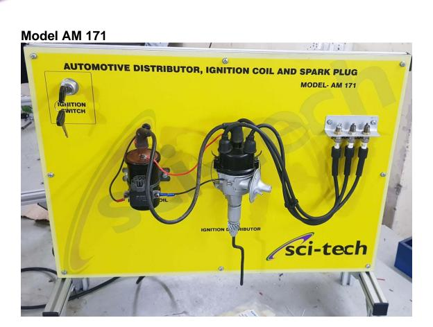
**Sci-tech Automotive Distributor, Ignition Coil & Spark Plug Model AM 171** demonstrates the operating principle and cross sectional view of distributor, ignition coil and spark plug.
